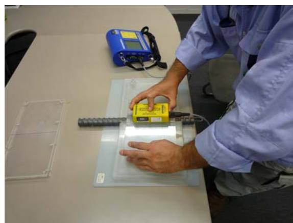
写真-2 かぶり厚さの測定誤差の検証状況 Photo2 Verification situation of measurement error of cover depth
